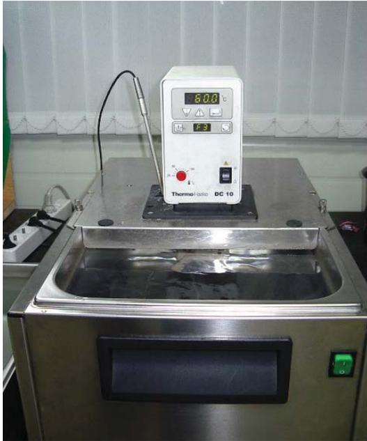
Picture on the left shows the Precision PID Temperature controller water bath for the Calibration Laboratory Standard.
